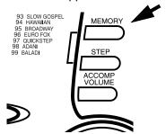
**Note: MEMORY** is a three-way switch. When you press it once, the keyboard enters the memory playback mode. When you press it again, it enters the memory record mode. When you press the button a third time, it turns off the memory function.
